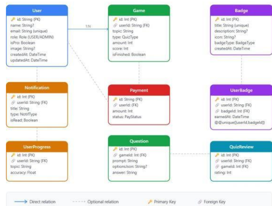
Fig. 3. Entity-Relationship diagram of the Quizmify Production database schema showing all 13 entities, primary keys, foreign keys, and cardinality relationships
