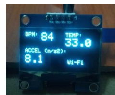
Fig 5.2: Upon supplying power, the OLED display initializes and displays the predefined startup information.
