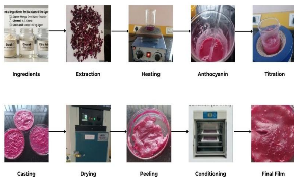
Fig. 2. Schematic of bioplastic film preparation via Solution Casting.
