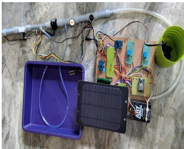
Figure 1(a): Hardware Prototype Development and IoT-Enabled Solar Drip Irrigation System.
