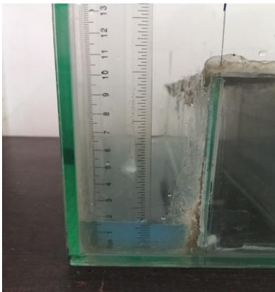
By using beach environment there is 1.6cm water over topping
