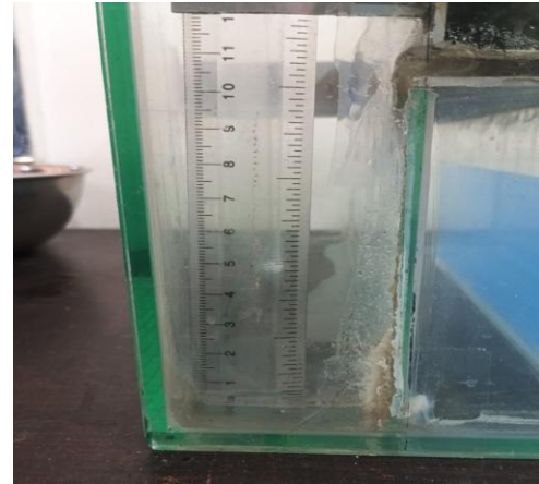
By using the step defence there is less over topping of water is 0.5cm
