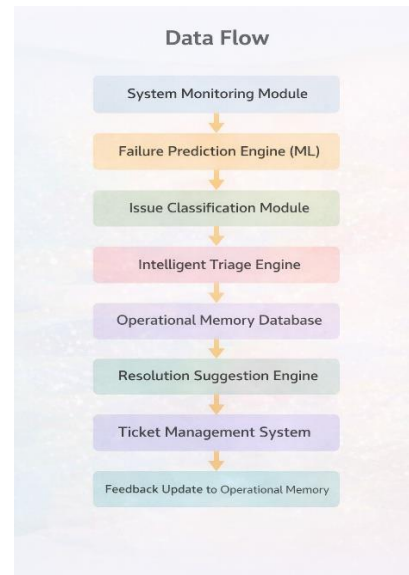
Figure 2: Data Flow of the Proposed Intelligent IT Support System
