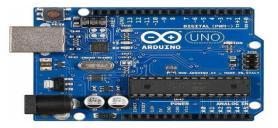
Operating at a system clock frequency of 16 MHz, the ATmega328P utilizes a Harvard architecture with separate program and data memories, enabling concurrent instruction fetch and data operations that enhance throughput and deterministic execution—critical for embedded control applications such as secure ration distribution systems.
