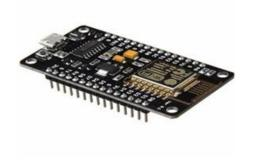
NodeMCU has SPI and I2C interface to enable the sensor communication and connection with it.
