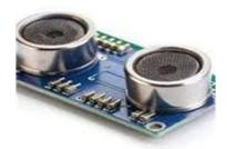
Ultrasonic sensor uses an acoustic wave generator to used to measure crop heights and can be used to monitor water and liquid levels.
