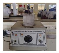
• Place 6 tablets in disintegration apparatus with water at  $37 \pm 2^{\circ}$ C.
