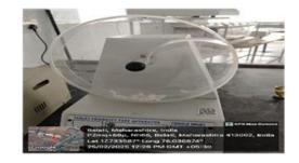
• Weigh 10 tablets (W1) and place them in a friabilator (100) revolutions at 25 rpm for 4 min).
