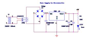
A power supply (sometimes known as a power supply unit or PSU) is a device or system that supplies electrical or other types of energy to an output load or group of loads. The term is most commonly applied to electrical energy supplies, less often to mechanical ones, and rarely to others.
