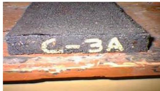
**Figure 2:** To Sample Beam C-3A with the Pave-Dry 381 Fabric.
