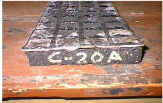
**Figure 1:** Uneven Coverage Using MS-1 Emulsified Asphalt Applied to Sample Beam C-20A with the HaTelit C40/17 Composite Product.
