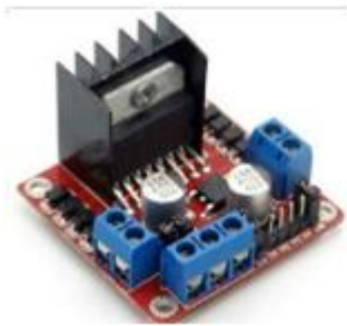
Fig:L298N Motor Driver
