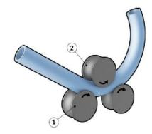
The rollers (or dies) play an important role in bending the pipes or sections. Firstly, the appropriate rollers or dies are chosen according to the type of section that to be bending then it is fixed to the shaft. Here three rollers (one with a high diameter and another two with similar and small diameters) are used.
