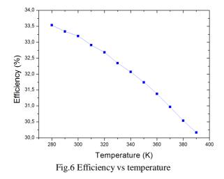
The variation of temperature with respect efficiency shows in the figure 5.4 it is obtained that efficiency decreases as the temperature increases this what obtain in the P-V characteristics of the solar panel where we that the panel will reach the optimum point at 25°C at the same time from the above graph that it will produce maximum efficiency at 300K (i.e.27°C)
