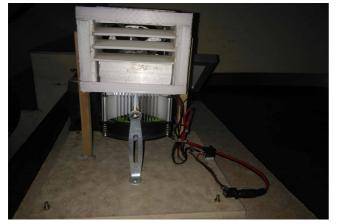
Fig.2 photographic view of peltier module
