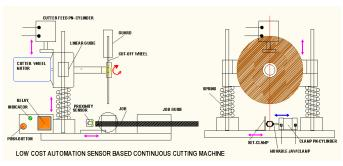
Figure 04: 2d Design of Semi-Automated Robotic System
