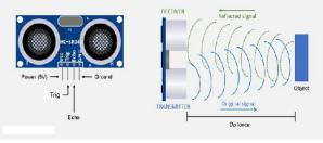
Fig.3.5: Ultrasonic sensor
