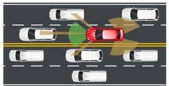
Fig.4.1: System scenario of V2V
