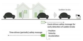
Fig.1.1: Collision avoidance using V2V communication
