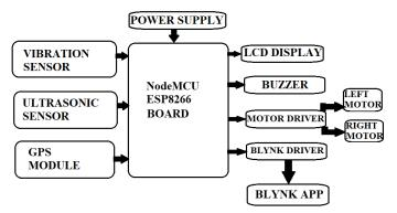
Fig.3.2: The proposed block diagram for vehicle-to-vehicle communication using IOT.
