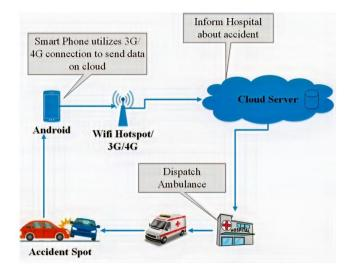
Fig.1.2: Accident Detection and Reporting System (ADRS)
