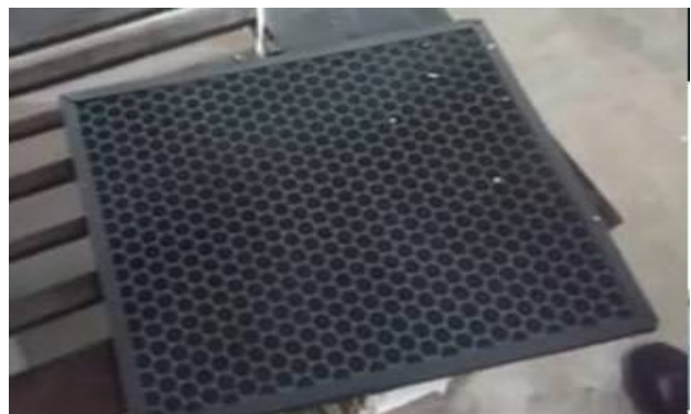
Fig 4: Carbon activated filter
