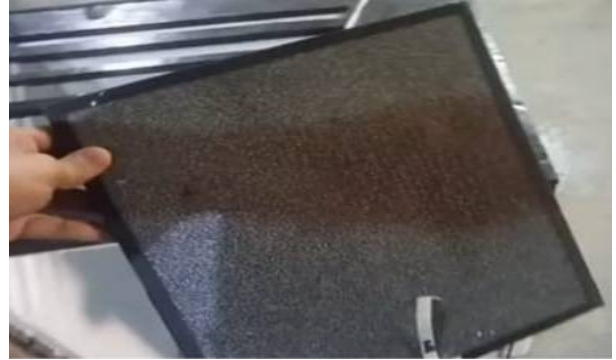
Fig 6: Photo catalyst filter
