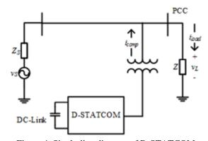
Figure 4. Single-line diagram of D-STATCOM
