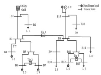
Figure 5. Single-line diagram of the 16-bus test system
