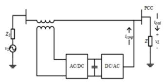
Figure 3. Single-line diagram of APC
