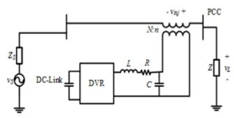
Figure 2. Single-line diagram of DVR
