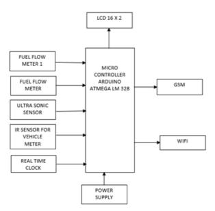
Fig. Block Diagram of Fuel data monitoring system
