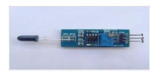
**Smoke sensor-** smoke sensor is used in this system. When an industry machine has an fault in system its produces an smoke and other gases. Its operate on an 4-5 v power.
