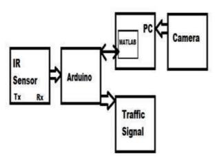
Fig. 1 Block Diagram for Traffic Monitoring System
