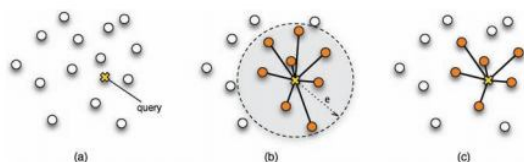
Fig. 1. Diagram of a typical query by content task represented in a two-dimensional search space. Each point in this space represents a series whose coordinates are associated with its features. (a) When a query is entered into the system, it is first transformed into the same representation as that used for other datapoints. Two types of query can then be computed. (b) A \epsilon -range query will return the set of series that are within distance \epsilon of the query. (c) A K -Nearest Neighbors query will return the K points closest to the query.
