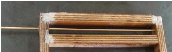
Figure 4: Mould for casting of single fiber
