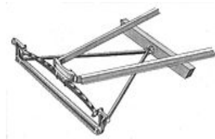
Fig: 1.6 Transverse Leaf Spring
