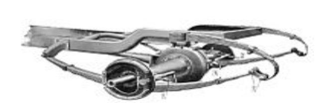
Fig: 1.4 Three quarter-elliptic Leaf Spring
