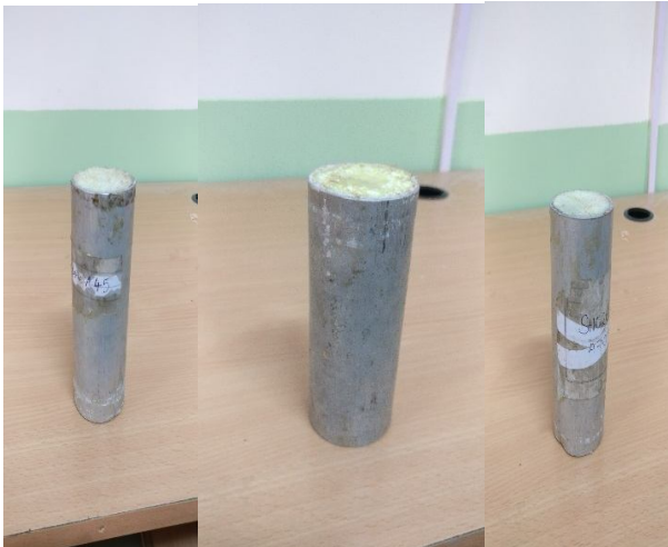
Fig 3:- Shore 45, 60 and 70 Elastomer filled annealed aluminium tube.
