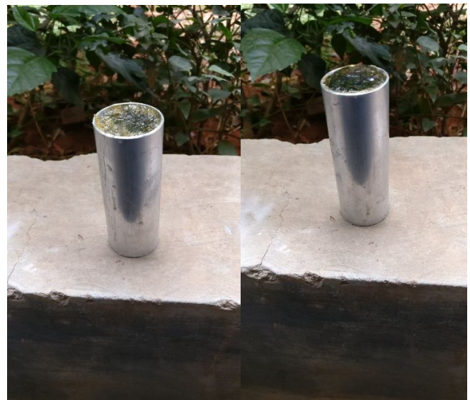
Fig 2:- Polyester and vinyl ester filled annealed aluminium tube.
