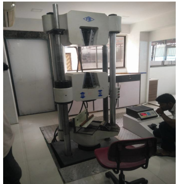
Fig.16. Test setup for GFRP material bracket
