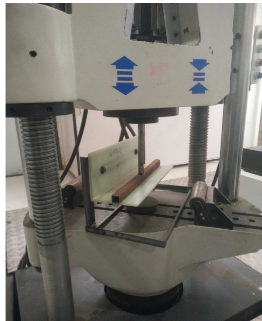
Fig.17 Compression loading of GFRP bracket
