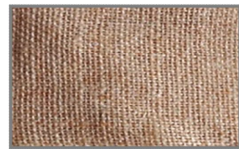
Fig.1 jute fiber woven mat (JWM)
