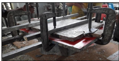
Fig.2 Fabrications of Composites laminates.
