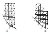
Figure 2.1. Hill building configurations: (a) Step back building; (b)Set back and Step back building
