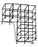
Figure 2.2. Building configurations at vertical cuts/steep slopes
