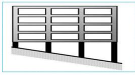
Figure 1: Building frame with short columns
