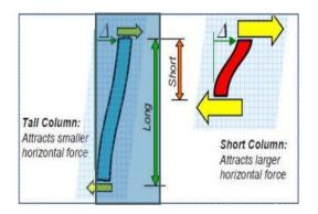
Figure 2: Structural behavior of short column under lateral load
