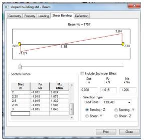
Fig: Column Share force bending moment diagram
