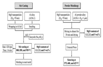
Flowchart representation of stir casting and powder metallurgy methods for fabrication of Al-MgO Nano composite
