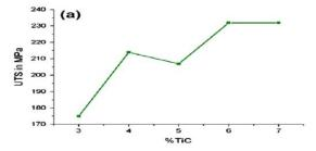
Effect of TiC addition on the mechanical properties of AMC. (a) Tensile strength
