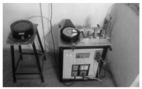
Pin-on-disc type tribo-setup.
