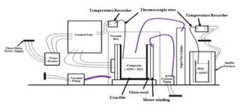
Schematic view of electromagnetic stir casting set-up
