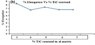
Effect of TiC addition on the mechanical properties of AMC. (b) Ductility.
