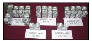
AMC castings produced with different percentage of TiC addition.
