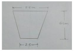
Fig.2 Photograph of Blade Dimensions
