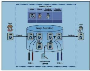
Fig 2: Architecture of Mirage Image Management System.
