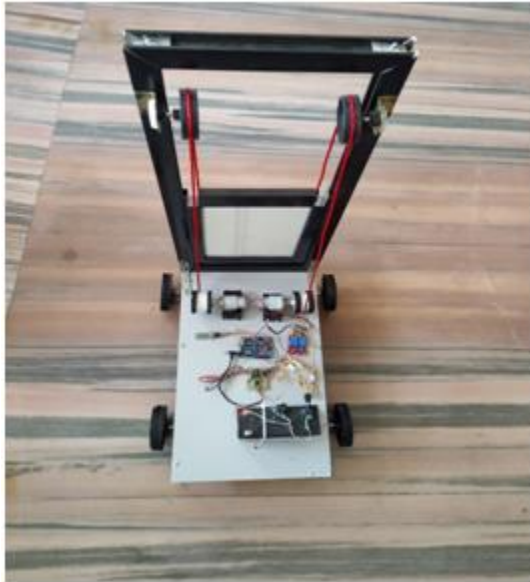
Fig.1-Final Model of Motorized Remote Control Mini Forklift Robot
