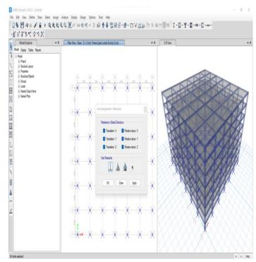
Fig 6 Assigning Fixed Support
