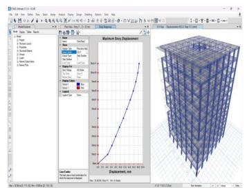
Fig 10 Storey Displacement
