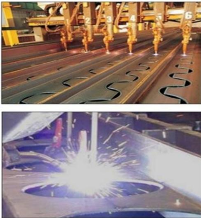
Figure2- Fabrication process flame cutting of hot-rolled profiles (Nseiret al. 2012).
