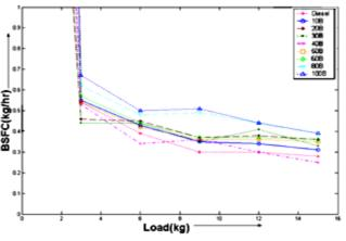
Fig. 5. Brake specific fuel consumption of cotton seed oil methyl ester, its blend and diesel with respect to load.
