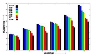
Fig. 9. HC emission of cotton seed oil methyl ester, its blend and diesel fuel with respect to load.
