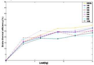
Fig. 4. Brake thermal efficiency of methyl ester of cotton seed oil, its blend and diesel with respect to load.
