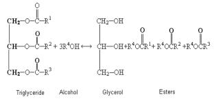
Fig. 1. Schematic representation of transesterification process.
