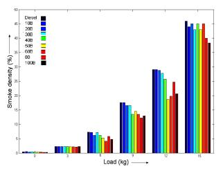
Fig. 12. Smoke density of cotton seed oil methyl ester, its blend and diesel fuel with respect to load.
