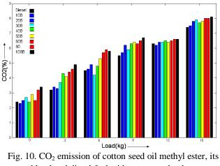
blend and diesel fuel with respect to load.
