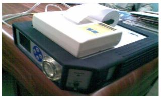
Fig. 3. Emission analyzer (AVL Digas 444).
