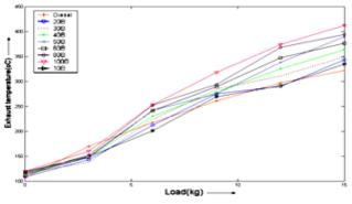
Fig. 7. Exhaust gas temperature of cotton seed oil methyl ester, its blend and diesel with respect to load.
