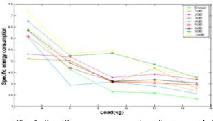
Fig. 6. Specific energy consumption of cotton seed oil methyl ester, its blend and diesel with respect to load.
