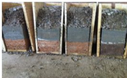
Plate 6 – Side view of the pavement models, the 1st on the left without geotextile and the rest with geotextile incorporated
