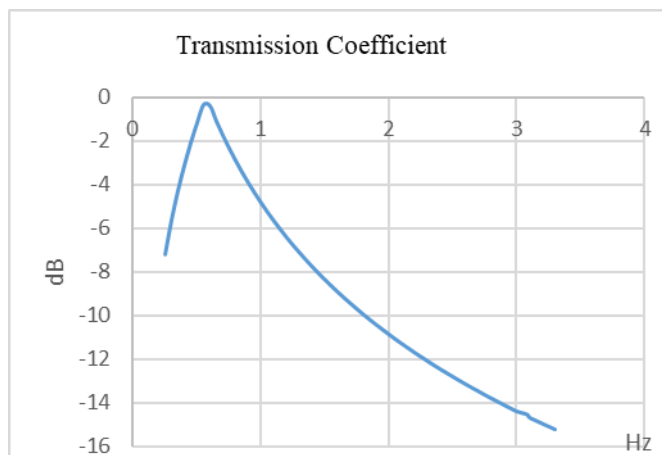
Fig: Transmission coefficient (S11) or Return Loss of proposed antenna
