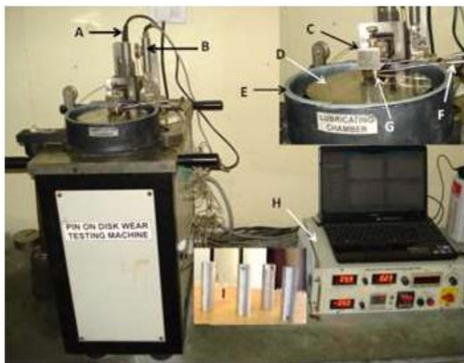
Fig. 4.2 Schematic diagram of the wear testing machine
