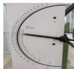
WITH OUT MACHINING: 12 JOULES
