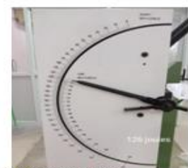
WITH MACHINING: 155 JOULES
