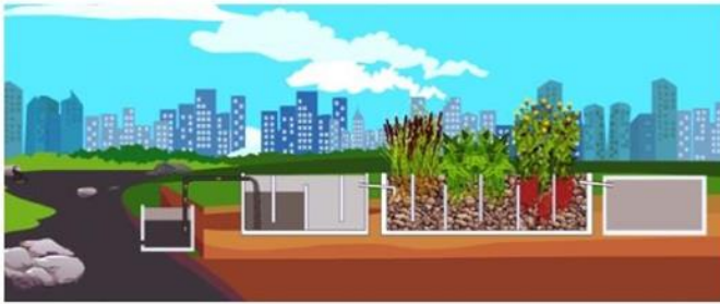
Fig. Cross sectional view of phytoremediation treatment system
