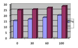
SPLIT TENSILE STRENGTH RESULTS for RA CONCRETE CUBES
