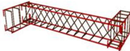
d) B4 - Inclined type Stirrups (45°)
