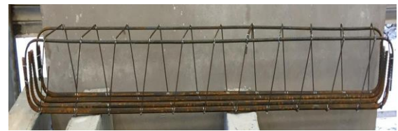
Fig. 1. Beam with continuous spiral reinforcement
