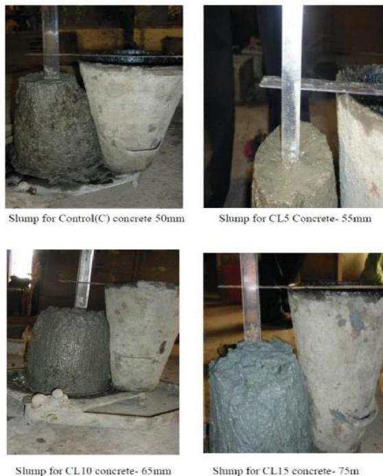
FIG: SLUMP CONE TEST
