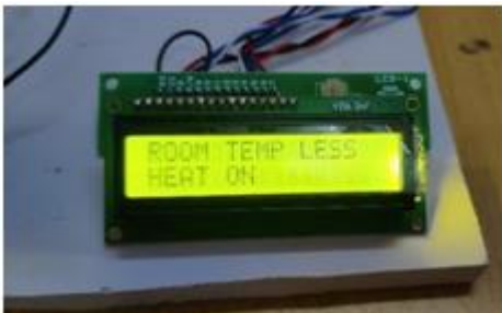
Figure 13: Room Temperature is Less, Turning on Heater
