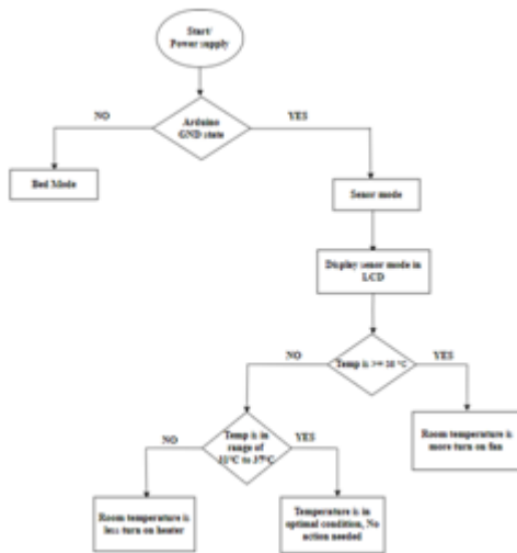
Figure 1: Flowchart of Temperature and Humidity of Surrounding
