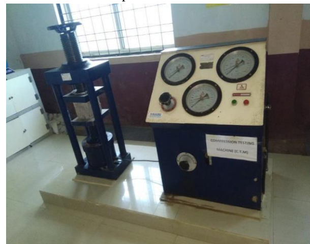
Fig 5.2: Compressive Strength Testing machine
