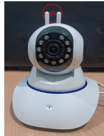
Figure 7: 360o Android App controllable Camera
