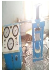
Figure 3.8: Compressive testing machine
