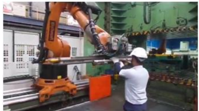
Fig:1 Manual gripper change process at die change time.
