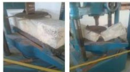
Fig.3.10 M25 Grade Concrete Flexure Test
