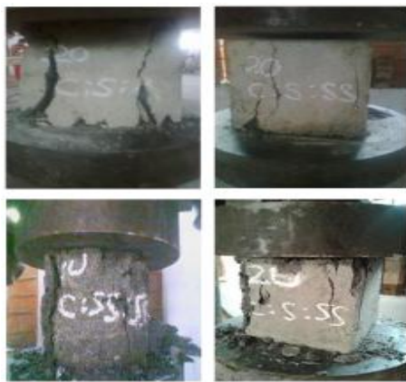
Fig 3.2 M20 Grade Concrete Compression Test
