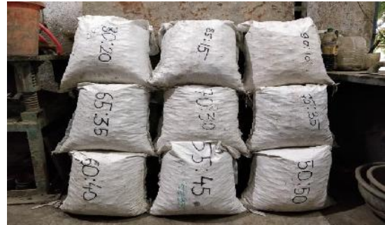
Fig 3.13 – Proportioning of 20 mm and 10 mm aggregate.
