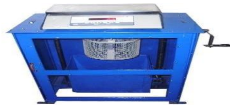
Fig–3.4 Coarse aggregatedensitytest set
