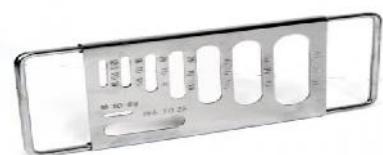
Fig – 3.9 Flakiness index test Instrument
