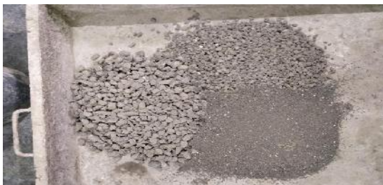
Fig 3.16 – Mixing of 20 mm, 10 mm and fine aggregate
